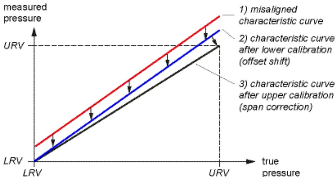
Figure 8: Effect of the upper and lower adjustment on the characteristic curve
