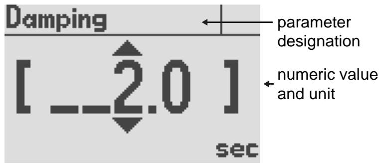
Figure 6: Elements when setting a numeric value
