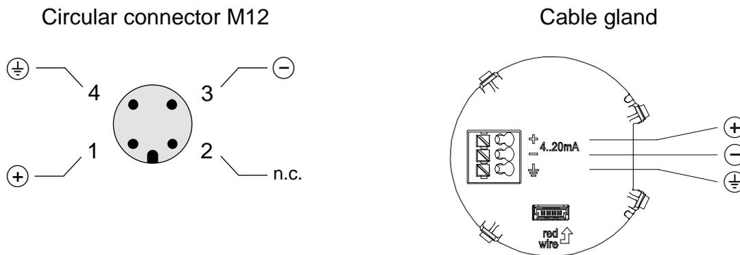
Figure 1: Options for the electrical connection
