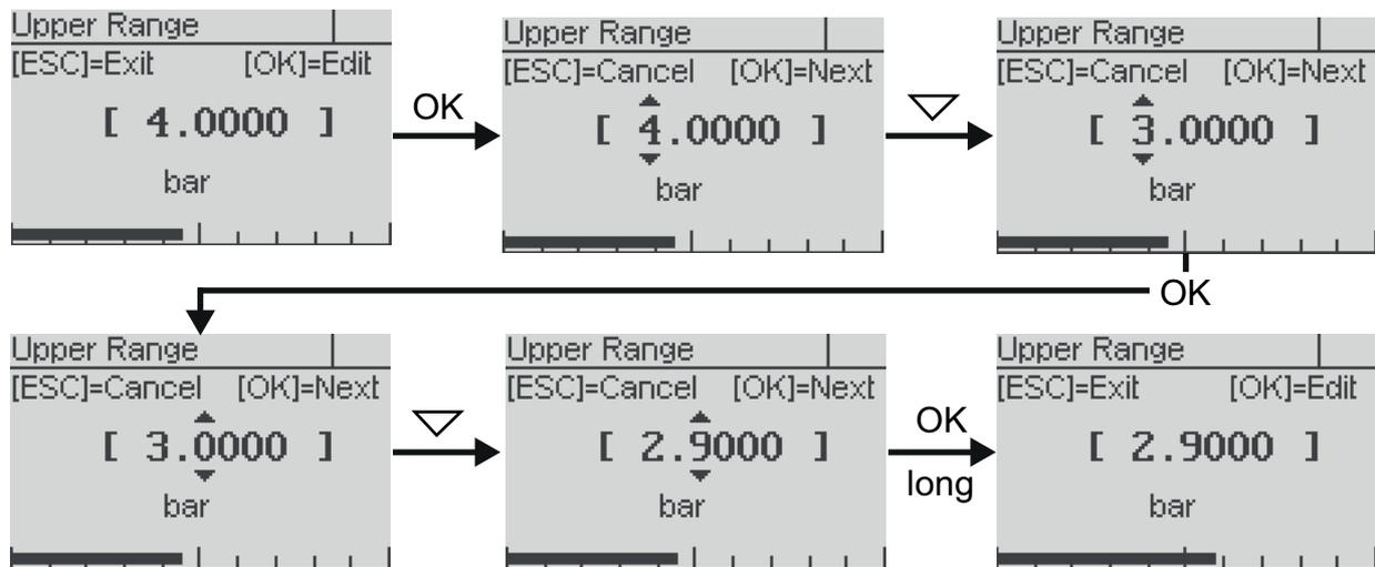
Figure 13: Procedure for number entry (e.g. changing from 4.0000 to 2.9000)
