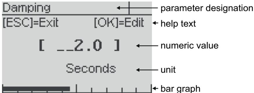
Figure 12 Elements when setting a numeric value
