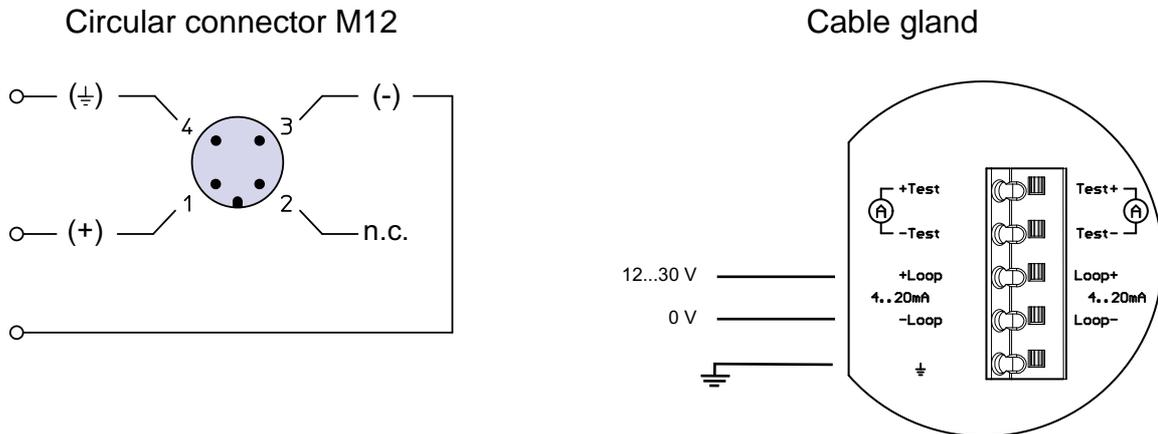
*Bild 1: Options for the electrical connection*
