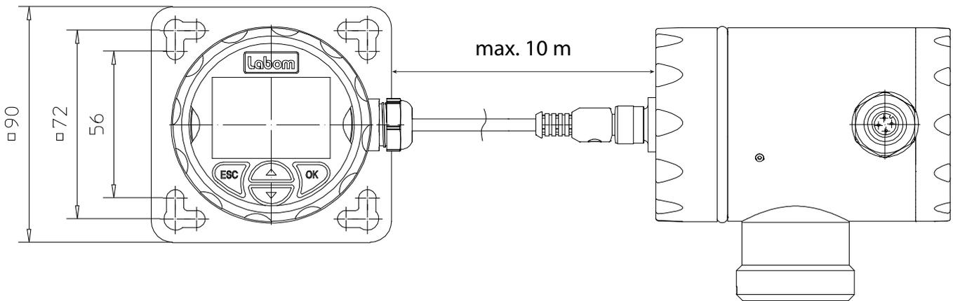
Figure 3: Remote display and control unit after installation
