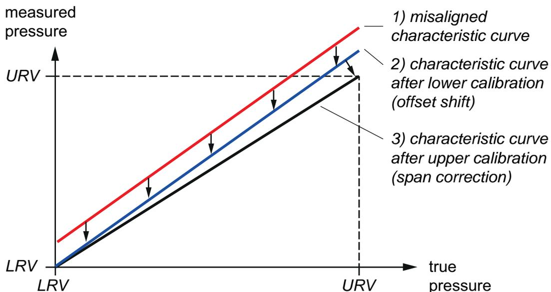
Figure 14: Effect of the upper and lower adjustment on the characteristic curve
