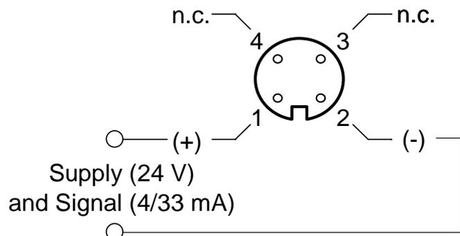
Figure 1: Pin assignment for M12 circular connector
