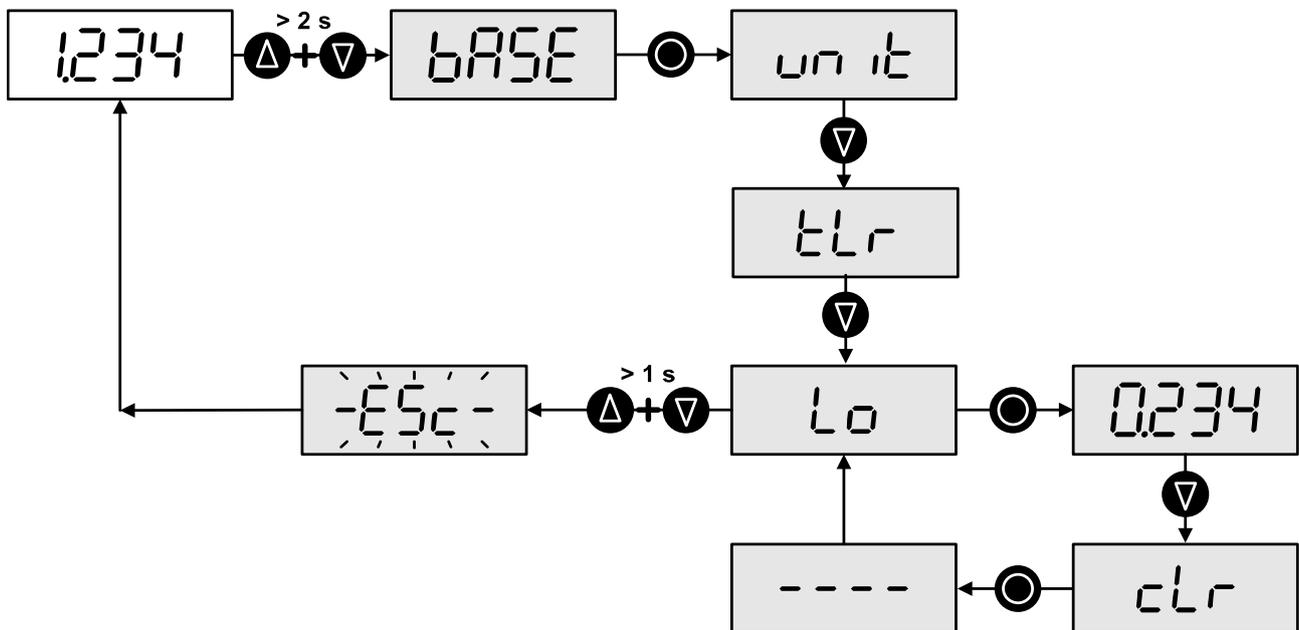
Figure 13: Operator actions to reset the minimum pointer
