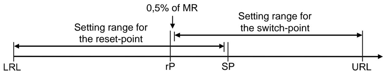
Figure 14: Setting ranges for switch-point and reset-point
