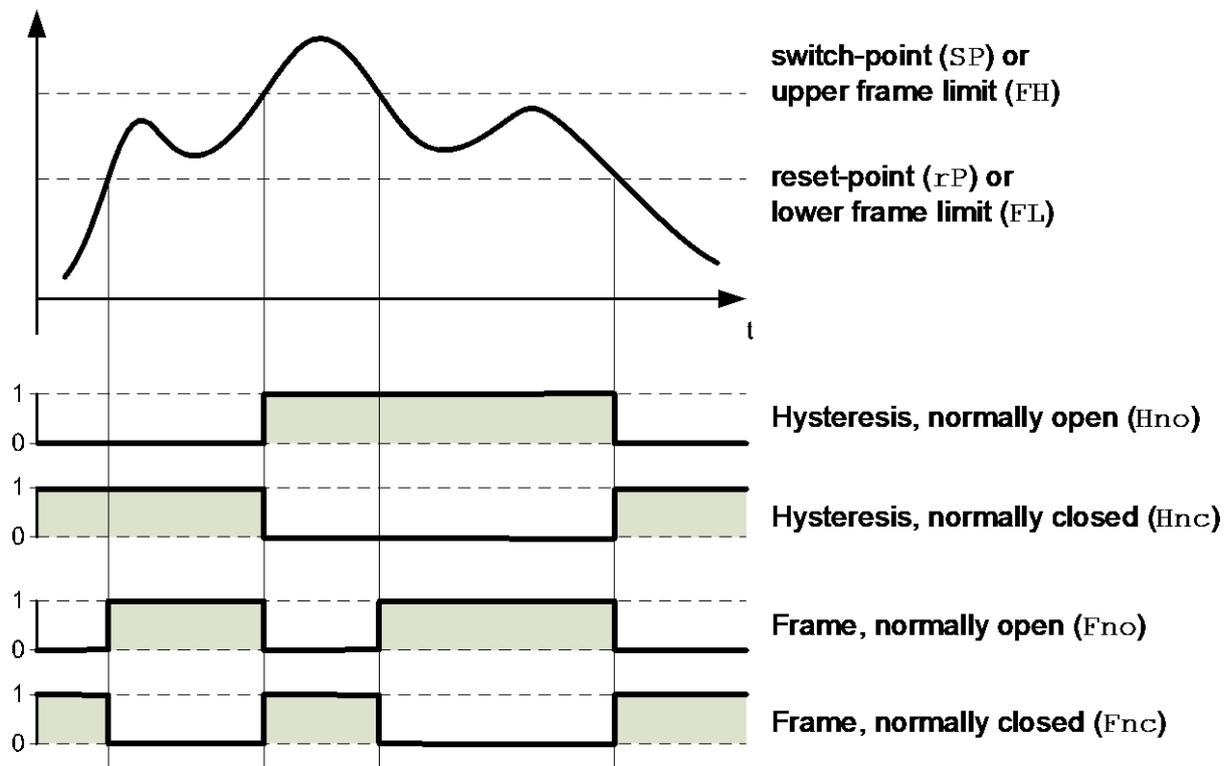
Figure 16: The output functions
