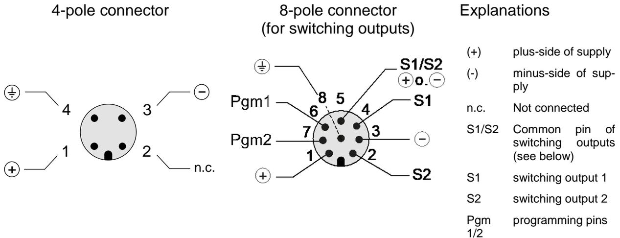
Figure 1: Pin assignment for M12 circular connector (device side)
