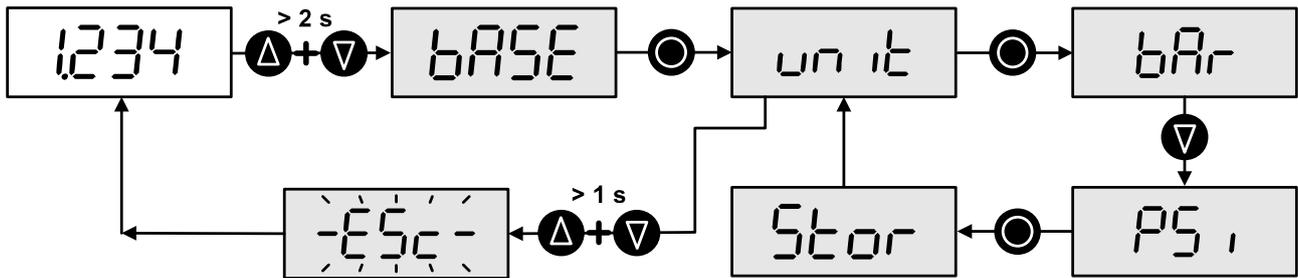
Figure 11: Operator actions for changing the measuring unit
