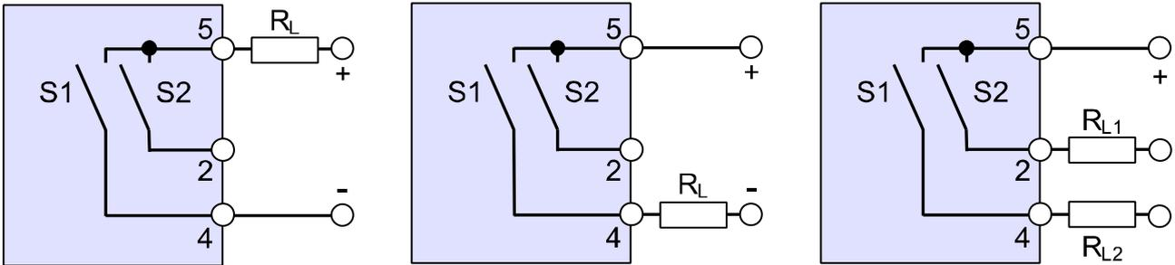
Figure 4: Connecting options with shared high-side (PNP/Highside)
