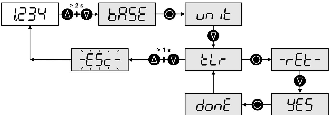
Figure 12: Operator actions for correcting the zero point
