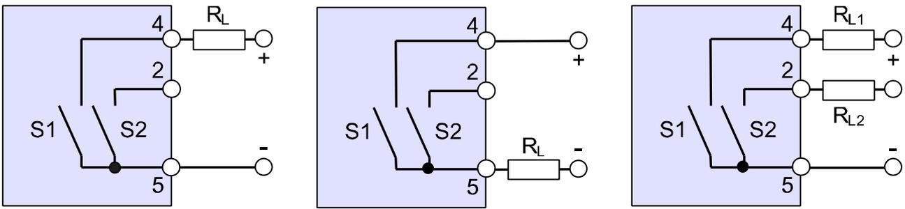
Figure 3: Connecting options with shared low-side (NPN/Lowside)
