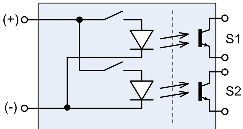
Figure 2: Switching outputs isolated from supply
