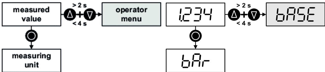
Figure 6: Button function in display mode, with example
