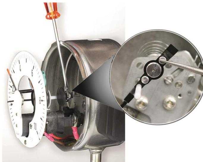
Figure 6: Zero-point correction
