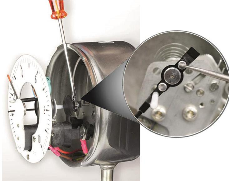
Figure 7: Zero-point correction
