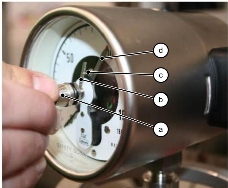
Figure 6: Setting the contact
