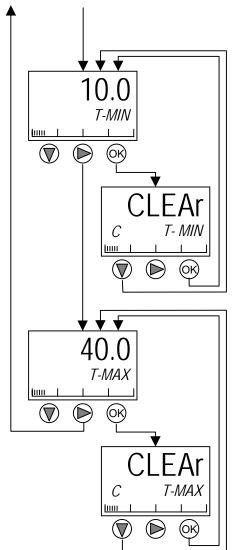
Display min-value (T-MIN submenu)
