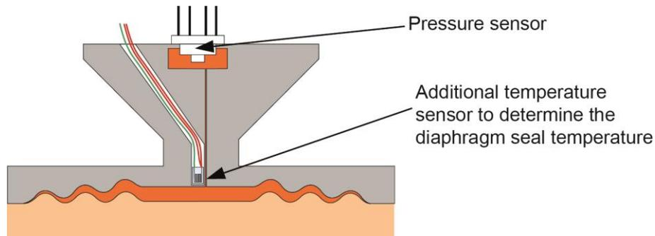
*Fig. 2 Positioning of the additional temperature sensor in the diaphragm seal*
