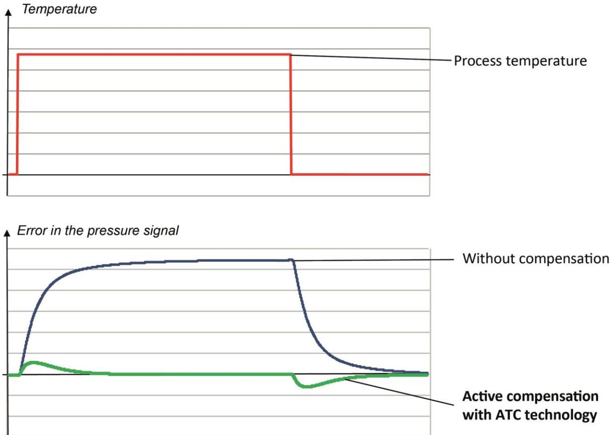
Fig. 3 Schematic comparison of a conventional system / system with ATC
