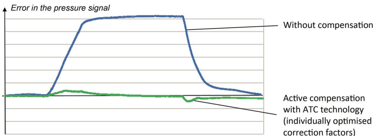
Fig. 4 Test measurement, comparison uncompensated with ATC compensation
