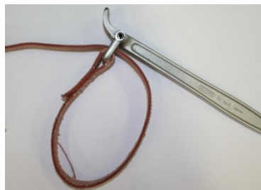
suitable tool: e.g. oil filter wrench with flexible strap
