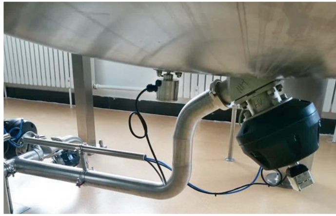
Fig. 1: Due to their small design, the combination of device and diaphragm seal has sufficient space underneath the tanks.
