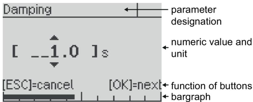
Figure 11: Elements when setting a numeric value
