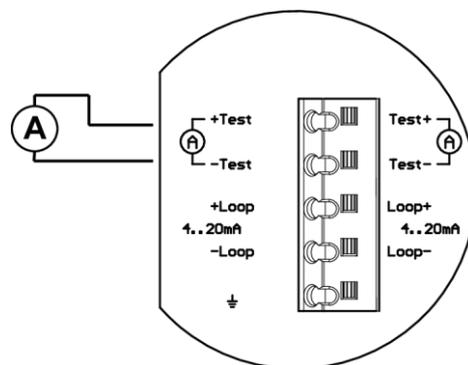
Figure 4: Current measurement during operation using test terminals
