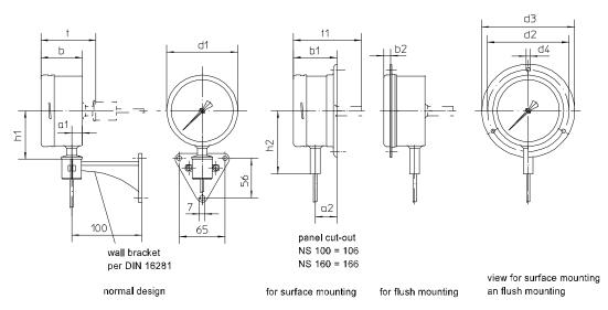
Temperature detecting element diameter d5, insertion length l1 and active length l2 see order details.
