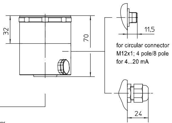
Instruments without LCD module come with closed cover
